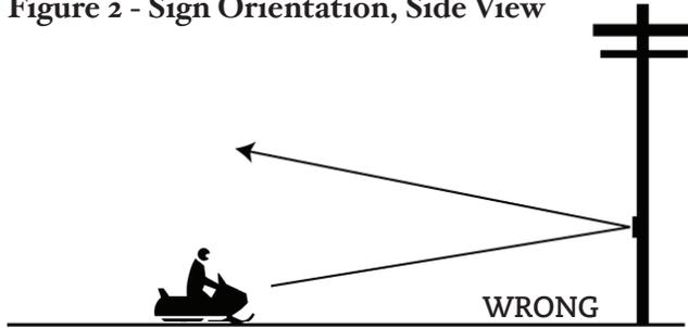
*Signs placed too high do not reflect headlight beams back to the rider.*
