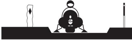
A single stake is used to augment an existing fixed object, such as a fence post. Note the use of the trail blazer on the post to provide a second reference point.
