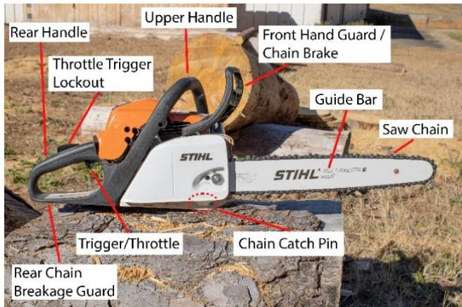
Figure 2: location of features on a chainsaw (Credit: Google)
