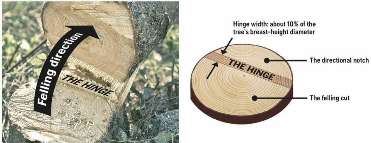
Figure 11: example hinge (credit: Husqvarna)
