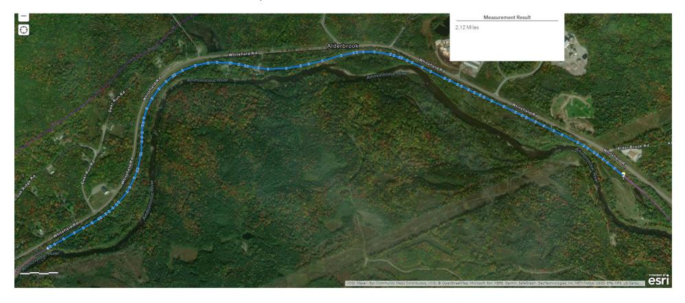
Close up of previous map showing end point of abandonment on trail. Do not remove any rails or ties beyond the endpoint marked on this map. At mandatory pre-construction meeting this location will be shown to contractor and marked in field.
