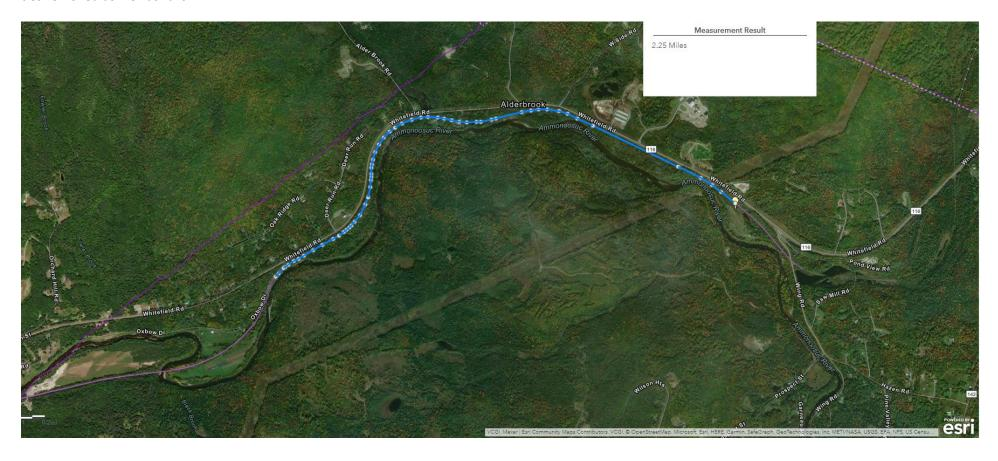
Map of 2.12 miles (11,230') of trail from Oxbow Dr. to a point close to Rt. 16 off of Wing Rd in Bethlehem. This is 650' shorter than previous section because 650' of rails were removed from Oxbow end but ties were left in place. This entire section needs both rail and ties removed.
