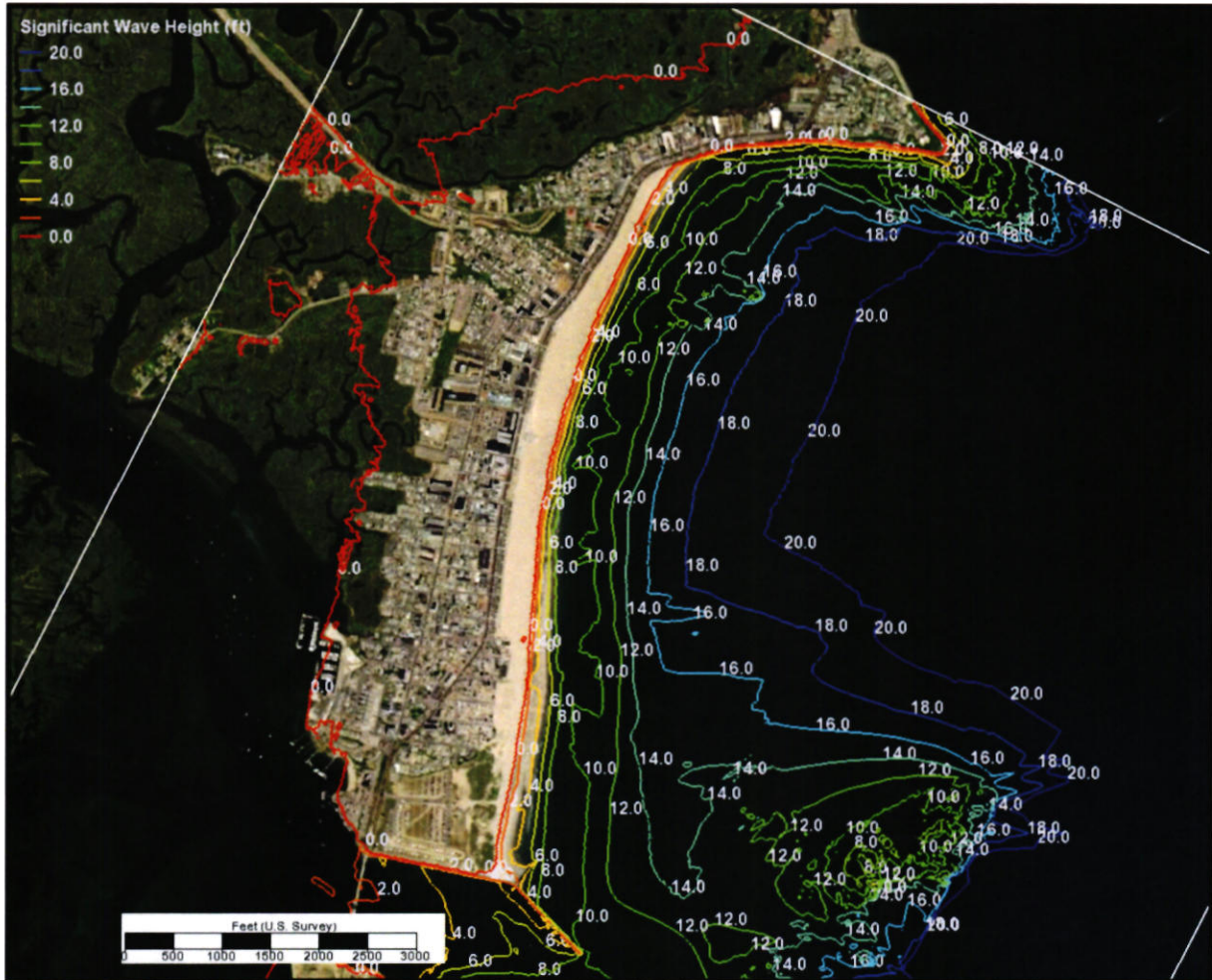
Fig. 16 – STWAVE Significant Wave Height Results for Present-Day Sea Level Conditions (ft)
